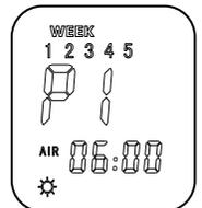
**Enter the system setting:** Press to switch on the thermostat when the unit is turned off. Within the next second please press Key as soon, you will enter into system setting. You can press to switch the system parameters. At the same time press or to modify settings. Select a set value. If you do not press the or , the parameters would not be modified. If you want to save the data, you must go through all the functions then exit the system menu.
