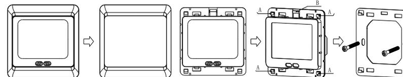
Step 1: Separate the Polycarbonate Bezel unit from the LCD screen.
